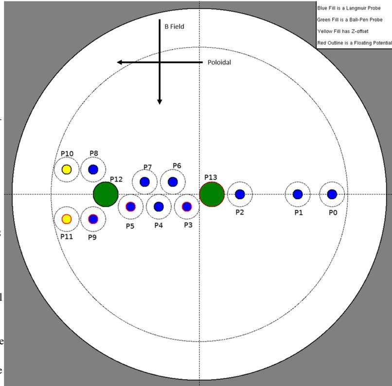
Along the poloidal axis there are several probes logarithmically spaced such that the scale resolution of turbulent modes is increased. Two BPP are located on the probe one biased, to measure plasma potential directly from equation (1). The other left floating allows an estimation of  $T_e$ .
