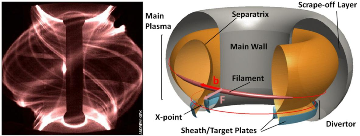
Figure (2): Left is a fast-shutter image of filaments in MAST. Right is a schematic showing a filament propagating in the SOL of a tokamak.
