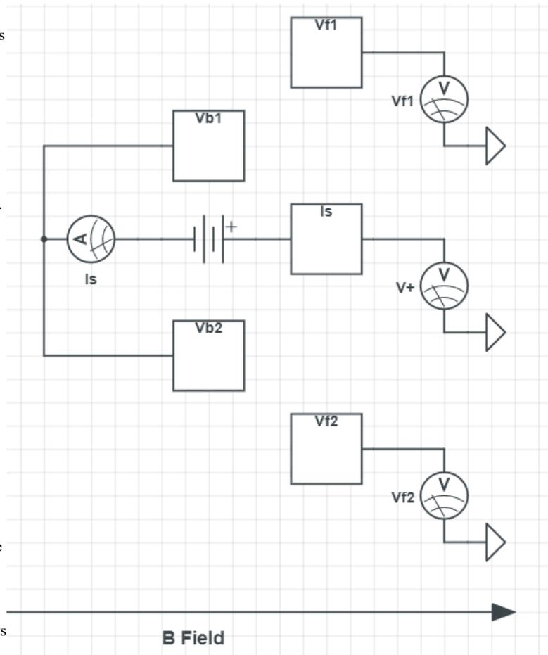
From this configuration, equation (3) thus becomes equation (5) as Tsui et al demonstrate [Tsui]. The layout is placed in such a way to reduce shadowing effects along the B field. The 5-pin balanced triple probe array can be used to measure the plasma potential, shown in equation (1). The array is placed tightly between the BPPs aiming to measure the same filaments allowing for a greater confidence in the measurements.
